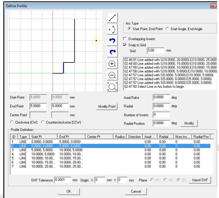
*Improvements to solid profile tool modeling capabilities in Third Wave Production Module 3D version 6.2 enables the software to better accommodate complex tool geometries.*
