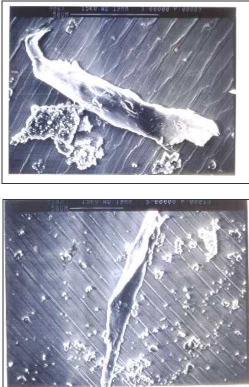
Figure 3: SEM images of chips for depth of cut =1\mu\text{m}
