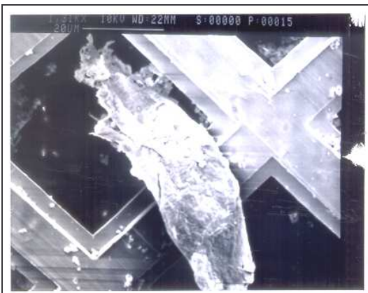
Figure 3: SEM images of chips for depth of cut =1\mu\text{m}
